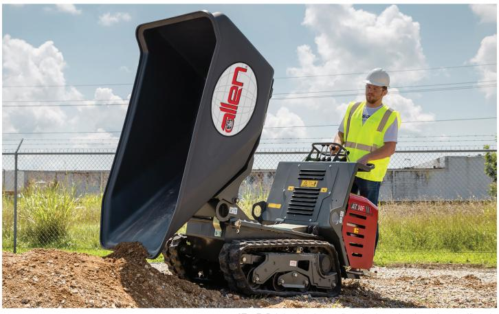
AT14F: Poly bucket design allows bucket to be cleaned more efficiently.
