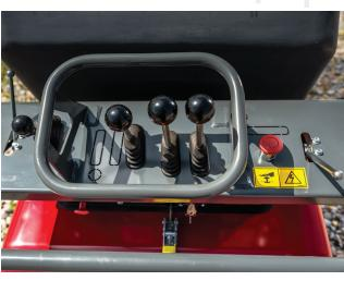
compact machine that will haul and dump any bulk material. This machine comes equipped with simple intuitive controls, a 20 hp engine, and a 14 cubic foot poly bucket. It is a perfect fit for concrete workers, landscapers, contractors or anyone else who needs to haul or dump material on a regular basis.
