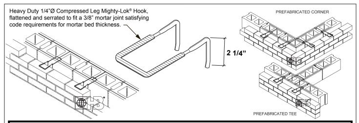
Hohmann & Barnard's Mighty-Lok Hook has been tested and designed to withstand over 290-lbf, in tension or compression, at maximum allowed offset (TMS 402/ACI 530 6.2.2.5.5.4) of 11/4" (disengagement of the pintle from the veneer anchor). These results exceed BIA recommendations and the capabilities of standard "round wire" hooks/pintles by over 100%, while maintaining the ASTM A1064/1064M wire specification.
