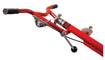
Fine pitch handles use a twist action to control blade pitch from flat to 28° and anything in between.
