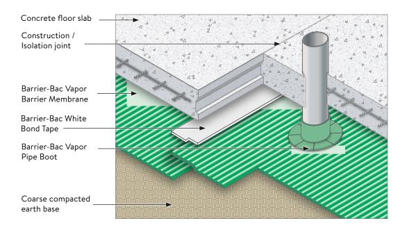
Step 5: Barrier-Bac Crawl Space Detail
